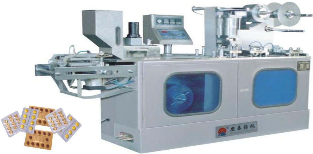
**The ideal blister packing machine for medium sized pharmaceutical factories. Equipped with micro-computer, touch panel operation, frequency speed inverter, adjustable stroke, ease of operation, high quality components, reliable and low maintenance; it is the ideal blister packer.**
